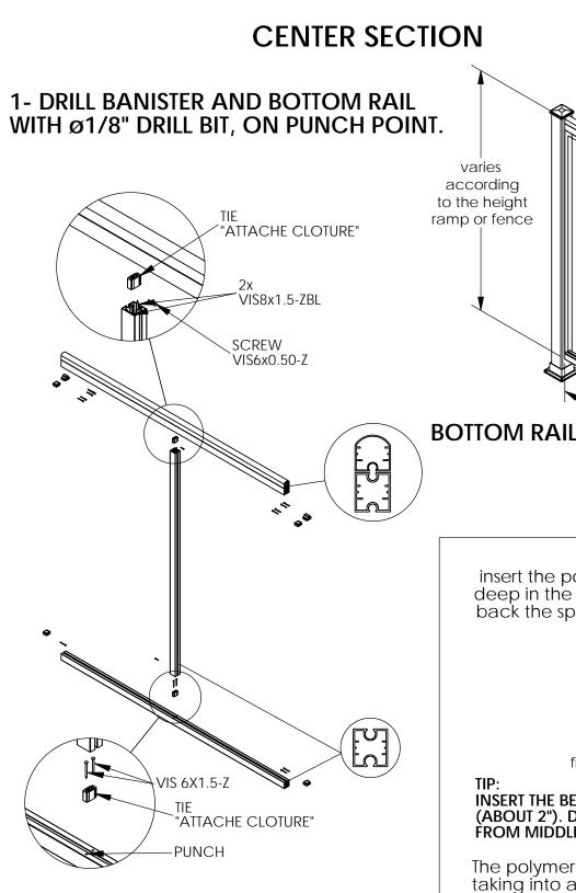
2- PUT A TIE ON THE BANISTER AND THE **BOTTOM RAIL WITH THE SCREW** VIS6-1.5-Z. JOIN THESE PARTS WITH THE UPRIGHT. JOIN THESE PARTS TOGETHER WITH THE SCREW.
