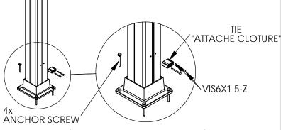
3- PUT TIES (ATTACHE CLOTURE) ON THE POST WITH THE SCREW VIS6-1.5-Z AT THE BOTTOM AND TIE "ATT90" WITH VIS8-1.5-ZBL ON TOP (SUPPLIED WITH CENTER SECTION) PUT THE END CAP
