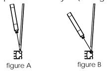
TIP: INSERT THE BEAD IN THE TWO SIDES OF A CORNER (ABOUT 2"). DO THE OTHER CORNERS, AFTER GO FROM MIDDLE TOWARD EACH CORNERS.
