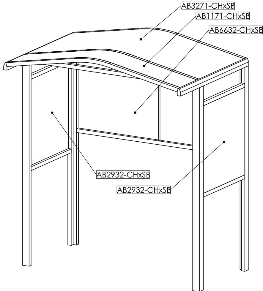
The polymer panels have been cut to fit, taking into account that they will expand when they are installed. Therefore, they may seem too small at first. If necessary, heat the polymer panel's surface equally using a hair dryer.
